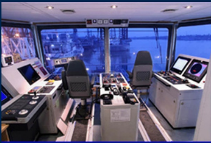
Wheelhouse AFT Console for Anchor Handling Tug Supply Vessel
