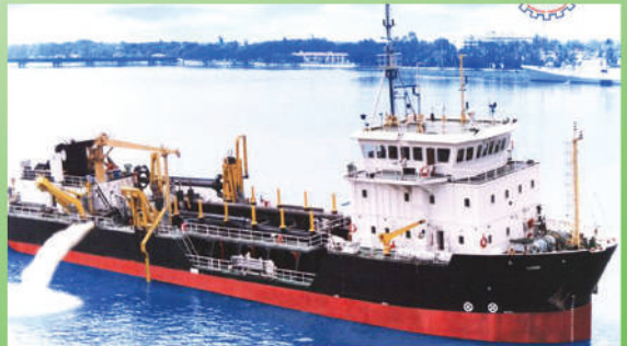
Trailing Suction Hopper Dredger 1700 Cu.M Capacity Designed & Built by Cochin Shipyard Limited for DCI Certified by IRS
