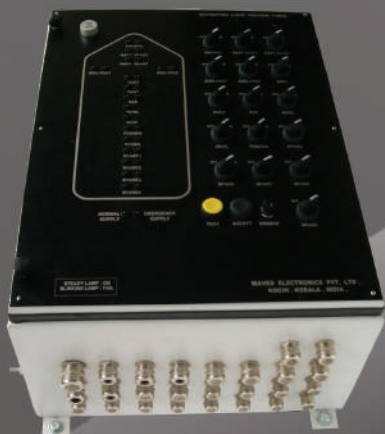
Relay Based NLCP Indian Navy (MO-Vizag) Project Certified by DGQA 600Hx450Wx275D
