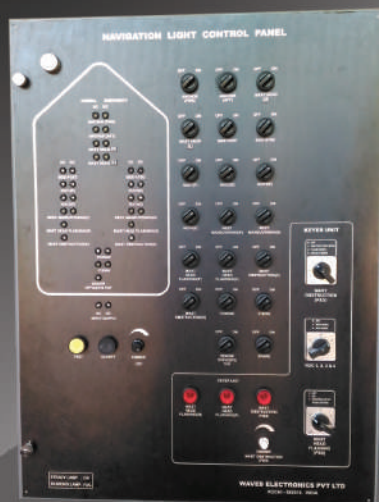
Microprocessor Based NLCP Indian Navy Landing Craft Unit Certified by DGQA 800Hx600Wx350D
