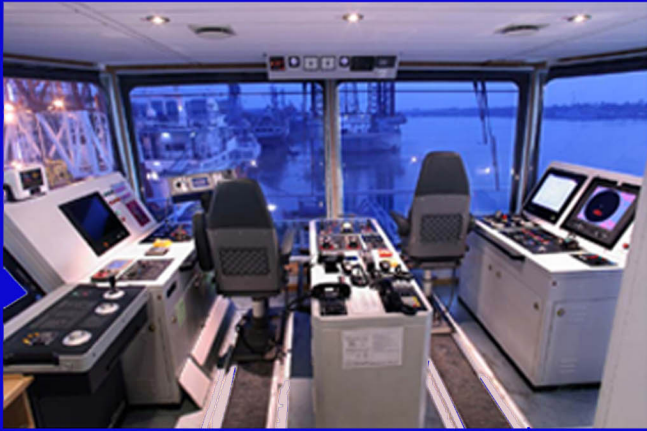
WHEEL HOUSE AFT CONSOLE OR 120T BP ANCHOR HANDLING TUG SUPPLY VESSEL ( SCI PAWAN )
